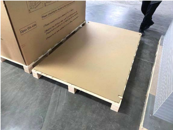
1. Prepare a pallet and back cardboard next to a fixed object (another pallet in this case)
