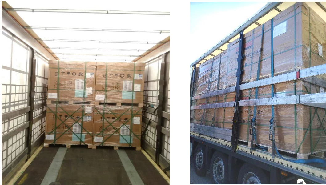
Image 1: Modules in the container/on the truck
